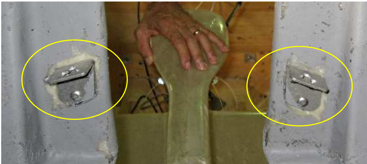
completed aileron cable mounts as viewed from the rear facing forwards
