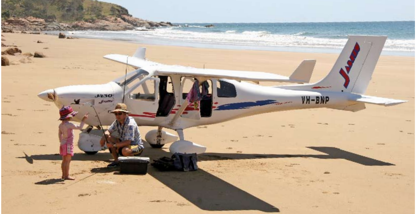
WEIGHTY ISSUES The Jabiru is manufactured using fibre reinforced plastic – much of the reason for its empty weight of 360kg. (Jabiru Aircraft)
