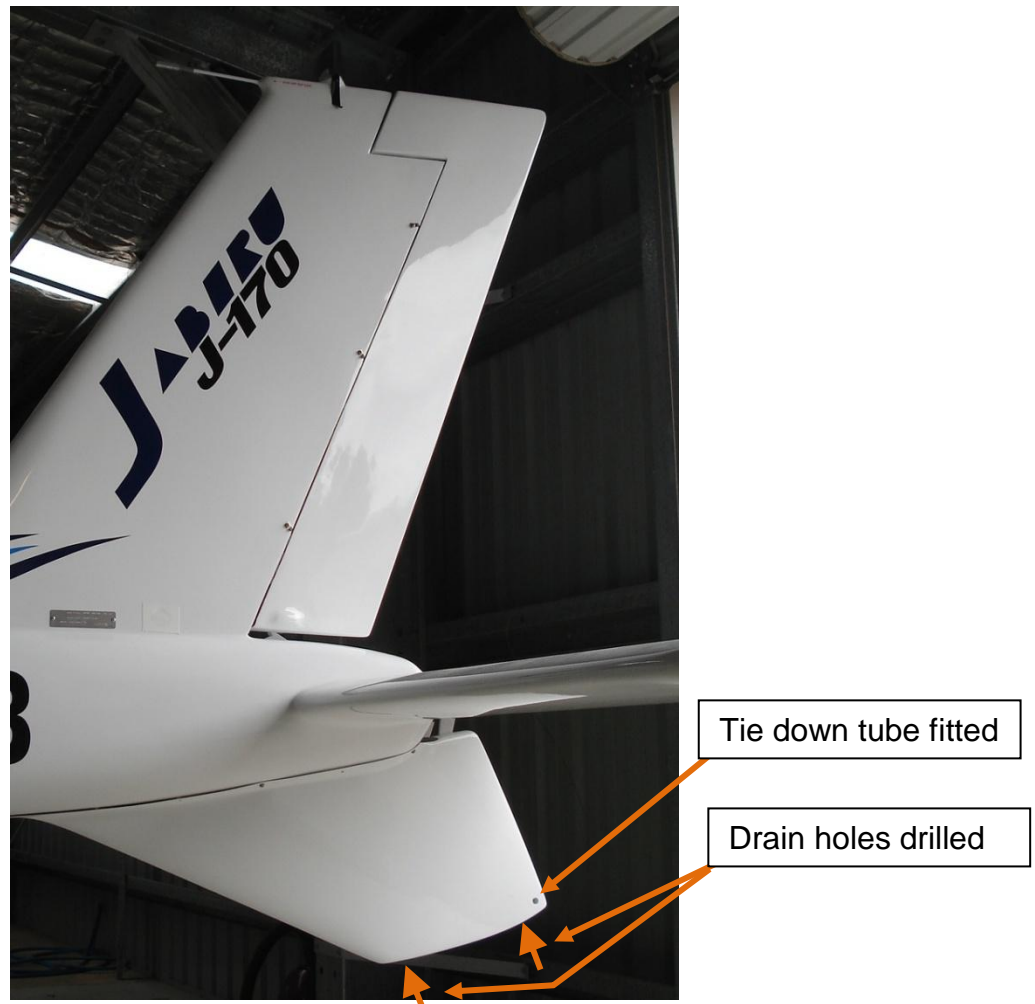
Figure 7 – New Ventral Fin Fitted
