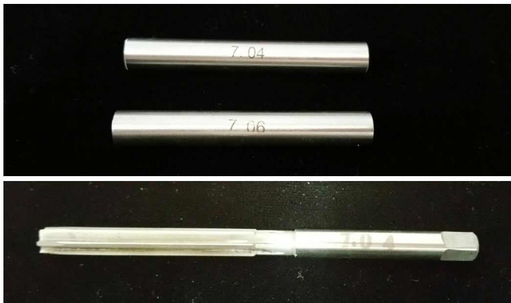
Figure 1: Valve guide Go-No go gauges and hand ream (available as a kit from Jabiru Aircraft)
