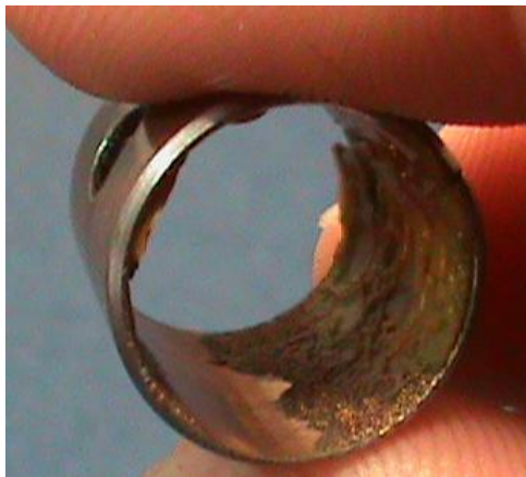
Figure 3: Badly worn rocker bush.
